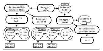
**Figure 3.** Truffle Mate's AST version of foo.bar(1) statement without including the field read node but with dispatch chains already filled. The bold circle nodes are metalevel nodes exclusive for Mate. Simple circled nodes were inherited from TruffleSOM.
