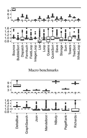
**Figure 4.** Overhead of TruffleMate normalized to Truffle-SOM, clustered by micro and macro benchmarks, without (above) and with (below) optimizations.
